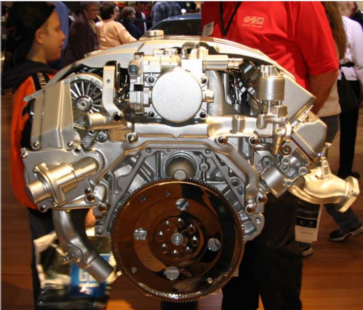
Buick's Northstar V-8 available in the Lucerne There was also a cutaway display for the 3.6 L V-6.
